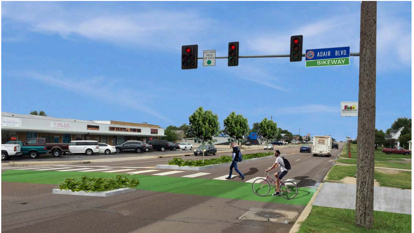
Above: The unused turn lane can be utilized as a pedestrian refuge with the addition of a landscaped median, increasing safety for bicyclists and pedestrians.
