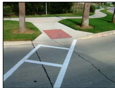
Illustration 6-5 STRIPING AT CROSSWALKS
