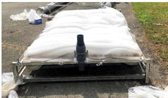
Image 3. Example WavTex Unit (front view) (Note - MWC flanged aeration scope break is different than shown)
