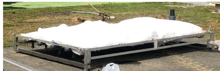
Image 4. Example WavTex Unit (side view) (Note - MWC flanged aeration scope break is different than shown)
